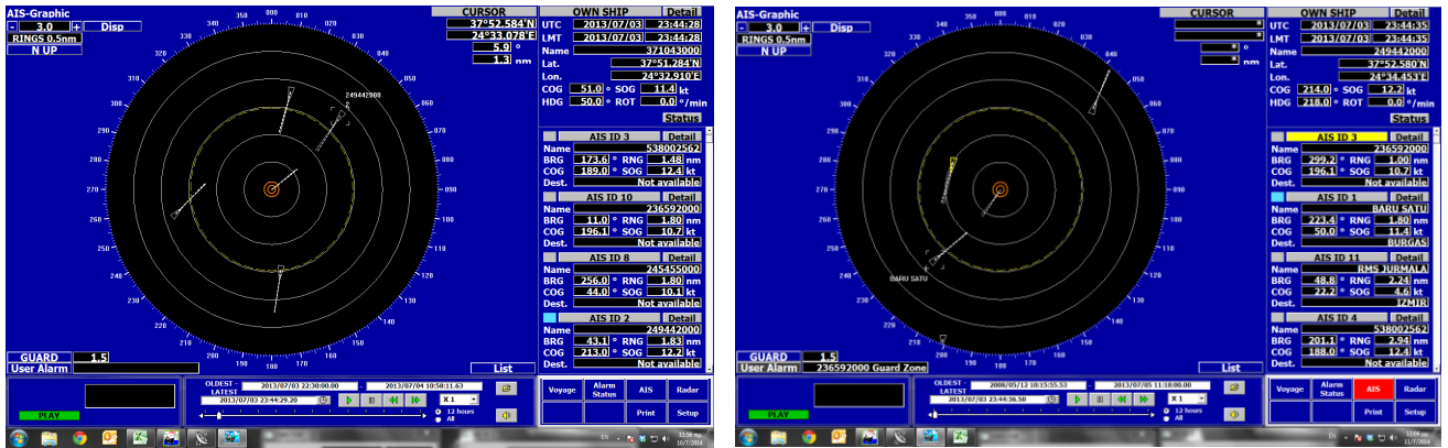
Pictures 4.2.2/1&2: Depiction of AIS feature of VDRs at the time when Baru Satu altered her course to port at 02:44:36.
